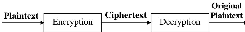
Figure (3.2) Encryption Process.
